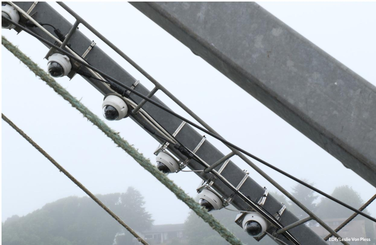
Fixed lens cameras affixed to the forward rigging of a bottom trawler.
