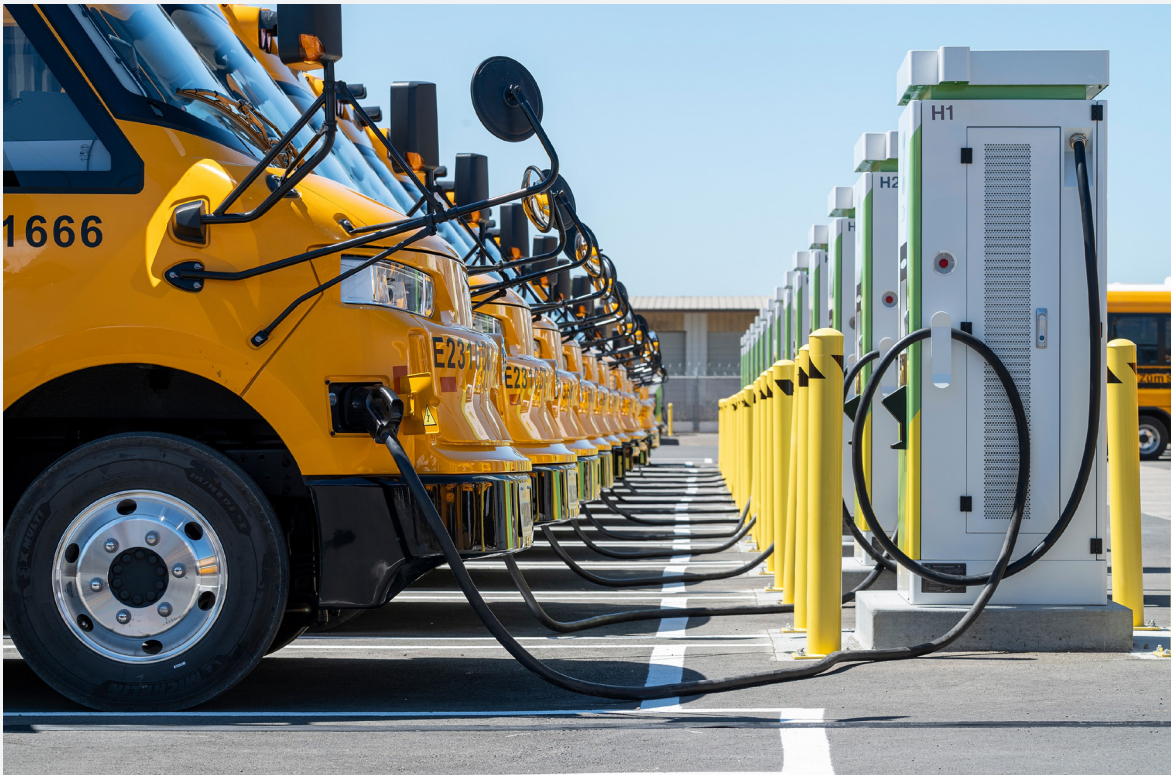
Virginia's virtual power plant pilot program will be able to aggregate devices, such as these electric school buses and their vehicle-to-grid charging systems, to dispatch power during peak demand. David Paul Morris/Bloomberg via Getty Images
