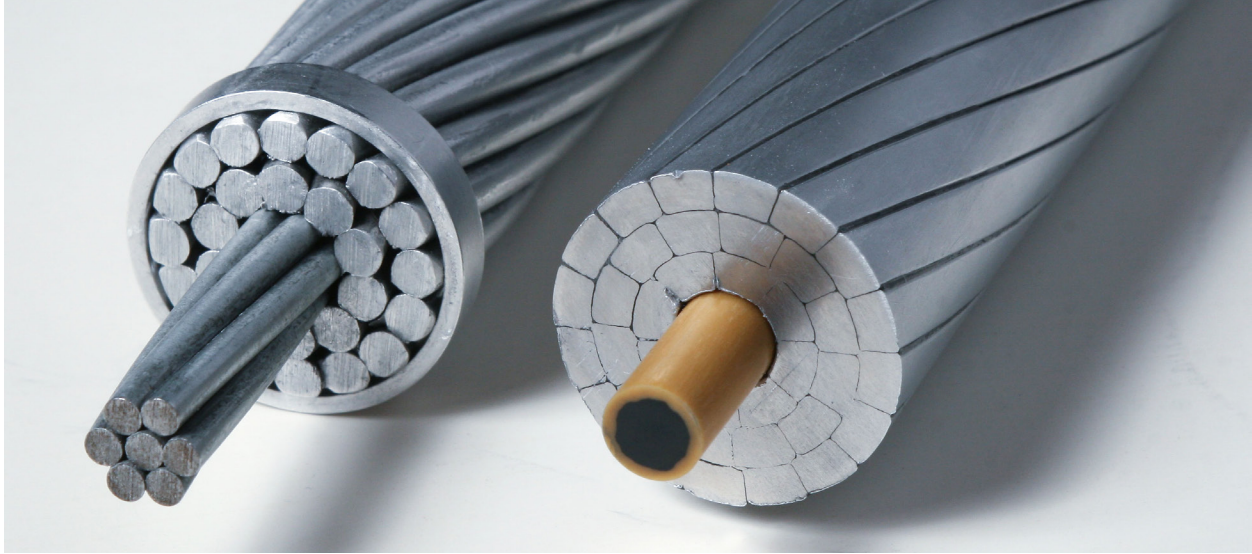
Two types of electric transmission lines. Advanced conductors (right) use more efficient and resilient materials to boost carrying capacity compared with conventional wires (left). If deployed nationwide, advanced conductors could quadruple energy transmission capacity in the U.S. and save $85 billion in systems costs by 2035, according to GridLab, a nonprofit energy use research organization. Courtesy of CTC Global
