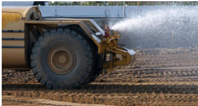
**Figure 15: Spraying water can reduce construction dust**
